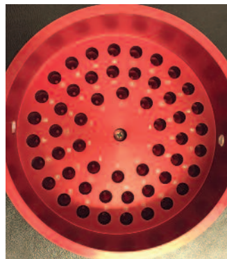
sample block holds up to 52 samples
